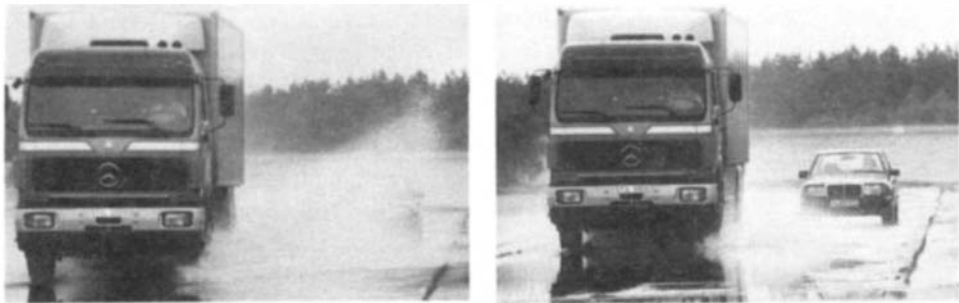
Figure 22 Splash and spray can be kept under a vehicle by shielding the non-steered wheels. (Left) Wheels uncovered; the passing car can hardly be seen. (Right) Wheels and sides shielded, as well as the rear of the truck. (Photos courtesy of Mercedes-Benz.)
